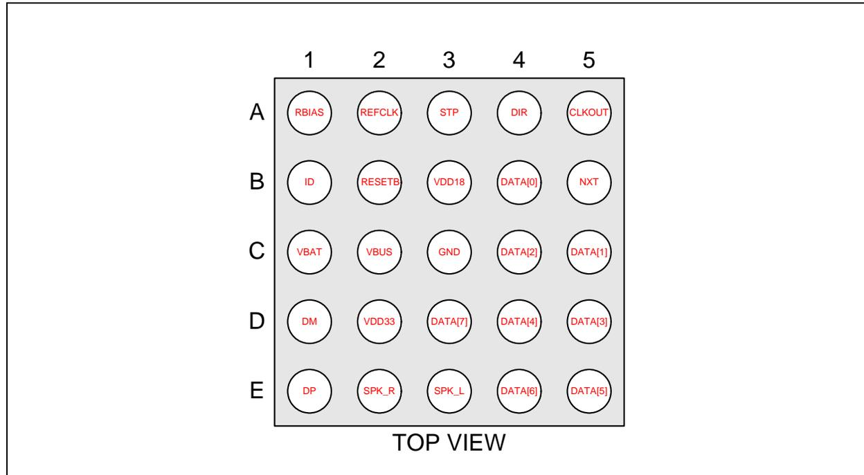
Figure 2 USB332x Ball Locations - Top View
