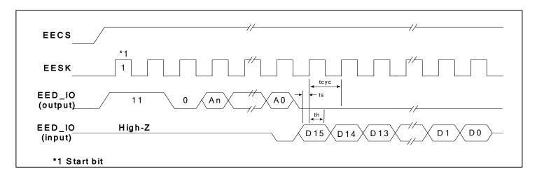
Figure 14. EEPROM Read Cycle Timing Diagram
