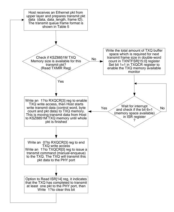
Figure 7. Host TX Single Frame in Manual Enqueue Flow Diagram
