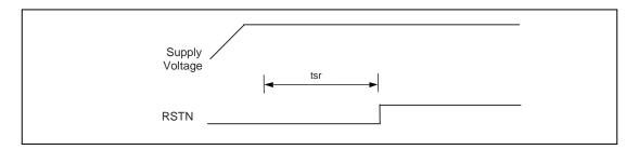
Figure 13. Reset Timing
