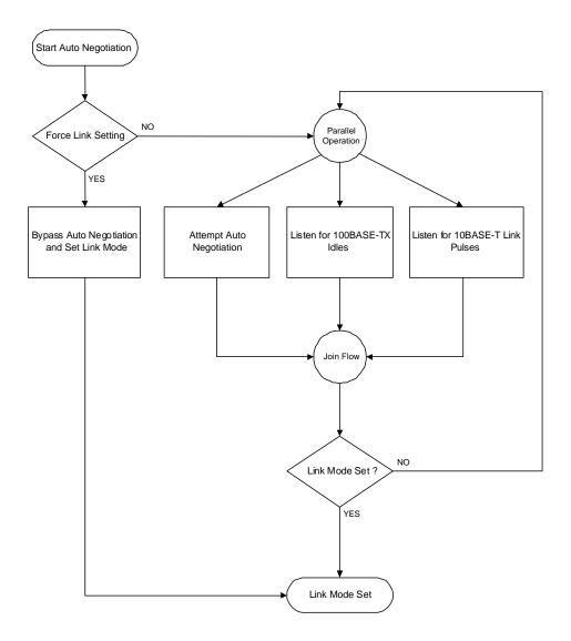
Figure 5. Auto Negotiation and Parallel Operation
