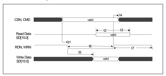
Figure 11. Asynchronous Cycle
