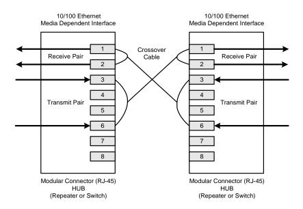
**Figure 4. Typical Crossover Cable Connection**
