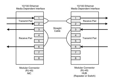
Figure 3. Typical Straight Cable Connection
