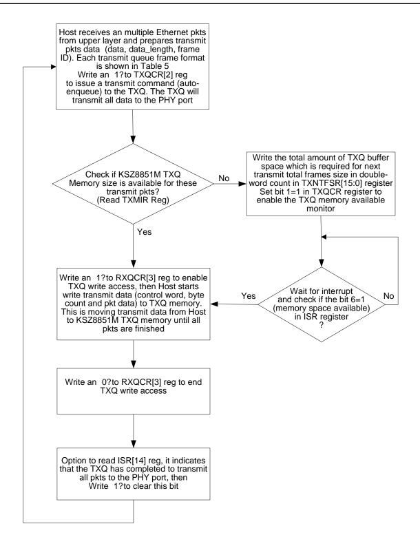
Figure 8. Host TX Multiple Frames in Auto- Enqueue Flow Diagram
