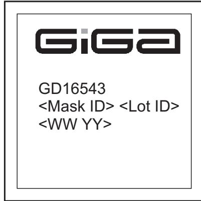
Figure 12. Device Marking, (Top - 48 pin and Bottom - 40 pin)
