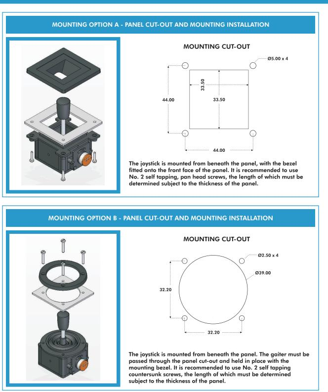
Note: During the mounting process, great care should be taken not to damage the gaiter. All panel cut-outs should be free from sharp edges and swarf that may damage the gaiter.
