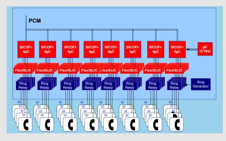
32-Channel Line Card High density linecard with centralized ring generator
