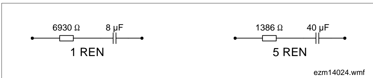
Figure 25 Typical Ringer Loads of 1 and 5 REN Used in US
