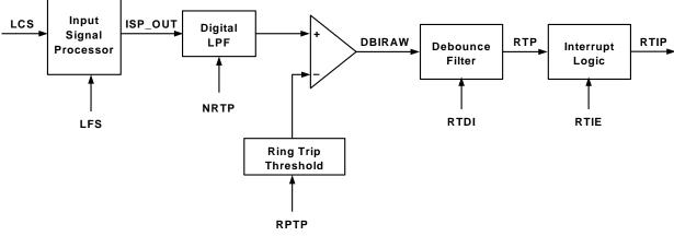
Figure 23. Ring Trip Detector
