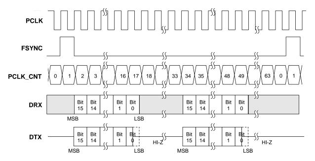
Figure 29. Wideband PCM Operation Example, Short FSYNC, PCLK = 512 kHz (TXS/RXS = 1)
