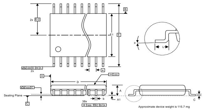
Figure 31. 38-Pin Thin Shrink Small Outline Package (TSSOP)
