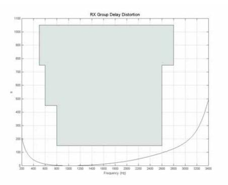
Figure 8. Receive Group Delay Distortion—Narrowband Mode
