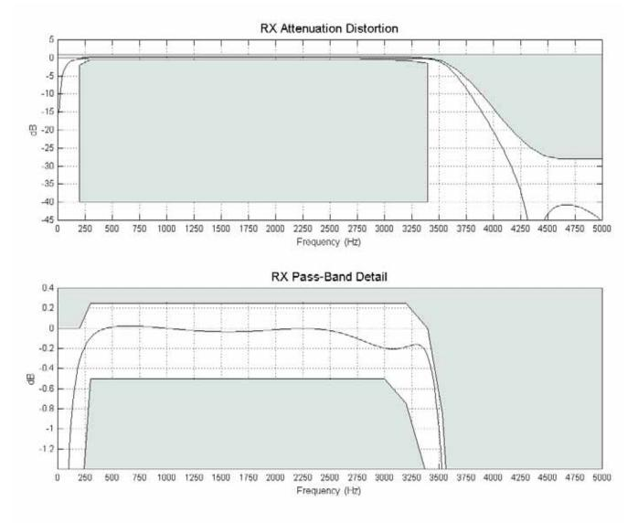
Figure 6. Receive Path Frequency Response—Narrowband Mode
