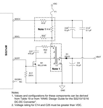
Figure 14. Si321xM MOSFET/Transformer DC-DC Converter Circuit
