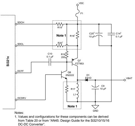
2. Voltage rating for C14 and C25 must be greater than VDC.
