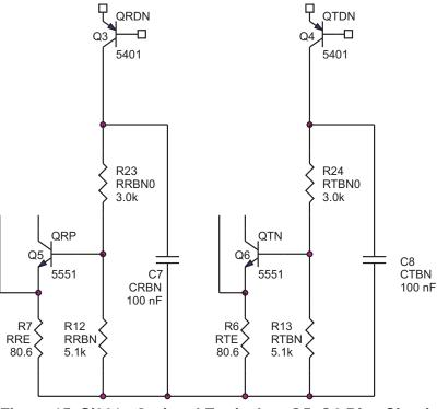
Figure 15. Si321x Optional Equivalent Q5, Q6 Bias Circuit
