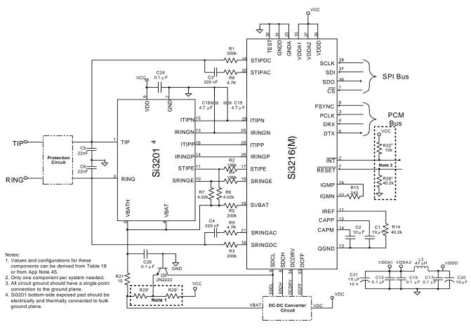
Figure 11. Si3216(M) Application Circuit Using Si3201
