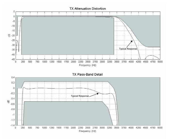
Figure 5. Transmit Path Frequency Response—Narrowband Mode
