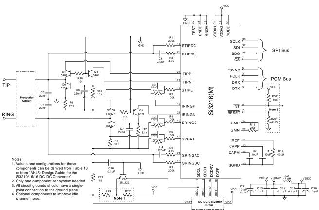
Figure 12. Si3216(M) Typical Application Circuit Using Discrete Line Interface Circuit
