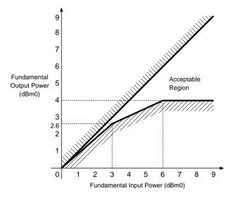
Figure 4. Overload Compression Performance
