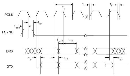
Figure 10. PCM Highway Interface Timing Diagram
