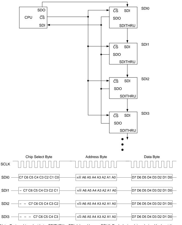
Note: During chip select byte, SDITHRU = SDI delayed by one SCLK. Each device daisy-chained looks at the LSB of the chip select byte for its chip select.
