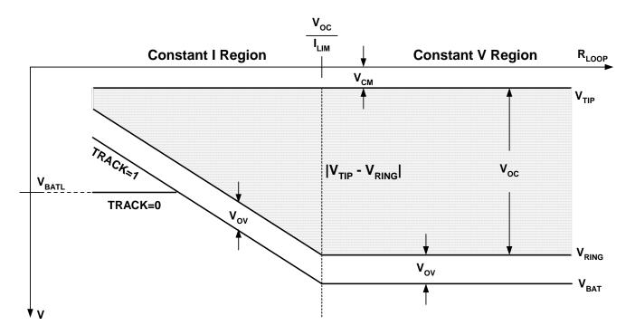
Figure 19.  $V_{\text{TIP}}, V_{\text{RING}}$  and  $V_{\text{BAT}}$  in the Forward Active State
