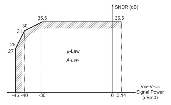
Figure 3. Transmit and Receive Path SNDR—Narrowband Mode
