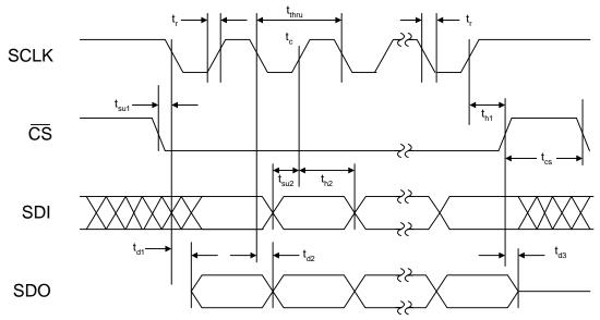
Figure 9. SPI Timing Diagram
