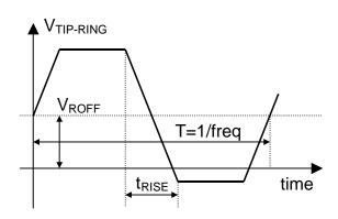
Figure 22. Trapezoidal Ringing Waveform
