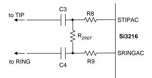
For 600 + 1  $\mu F,\,R_{ZREF}$  = 12 k $\Omega$  and C3, C4 = 100 nF For 900 + 2.16  $\mu F,\,R_{ZREF}$  = 18 k $\Omega$  and C3, C4 = 220 nF
