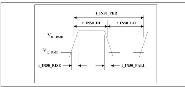
Figure 26 REFCLK Input Timing
