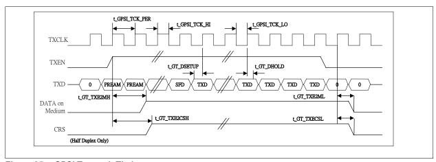
Figure 35 GPSI Transmit Timing
