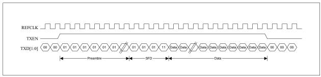
Figure 10 100M RMII Transmit Diagram
