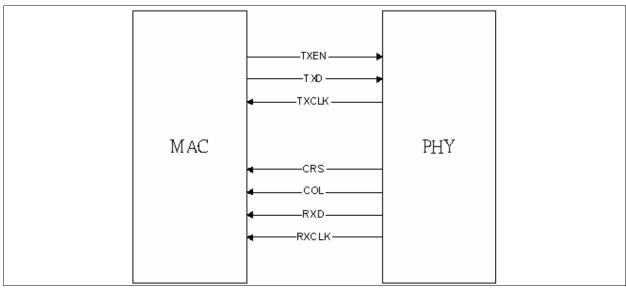
Figure 18 GPSI Signal Diagram
