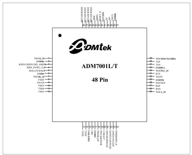
Figure 2 Pin Diagram
