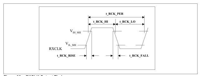
Figure 30 RXCLK Output Timing
