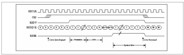
Figure 15 MII Receive With Symbol Error(100M Only)
