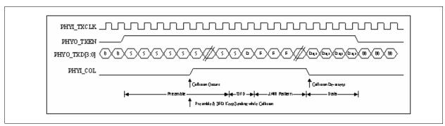
Figure 17 MII Transmit with Collision (Half Duplex Only)
