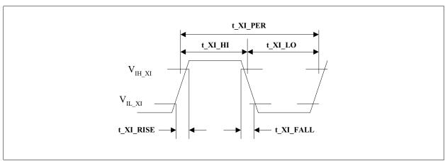
Figure 25 Crystal/Oscillator Timing
