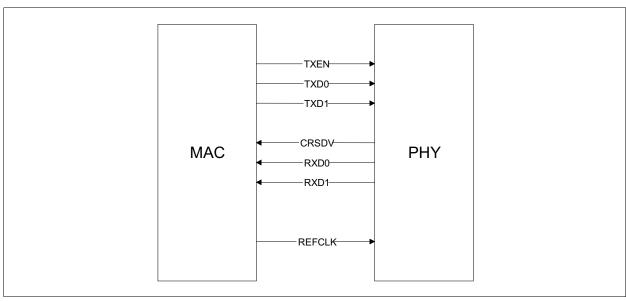
Figure 5 RMII Signal Diagram
