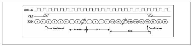
Figure 19 GPSI Receive Diagram
