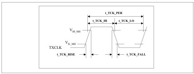
Figure 32 TXCLK Output Timing
