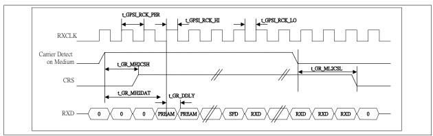
Figure 34 GPSI Receive Timing
