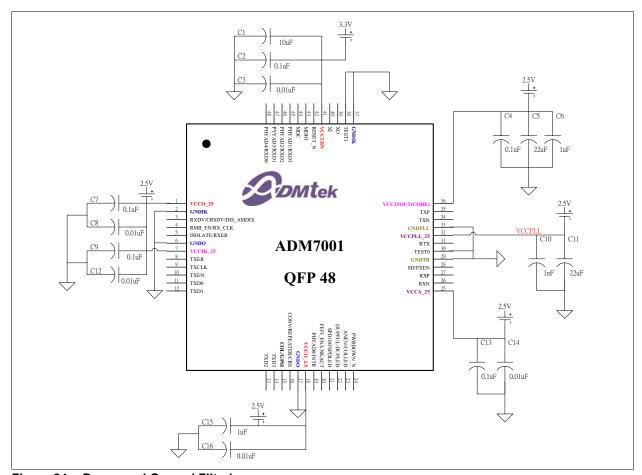
Figure 24 Power and Ground Filtering
