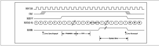
Figure 14 MII Receive With False Carrier
