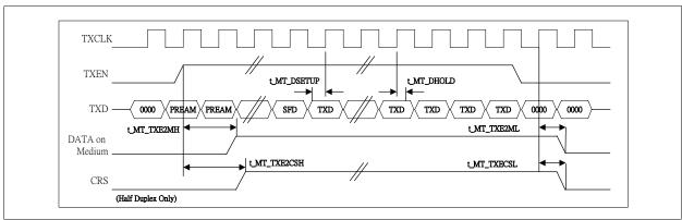
Figure 33 MII Transmit Timing
