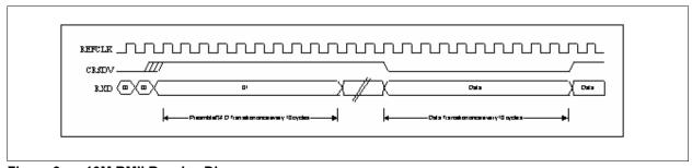
Figure 9 10M RMII Receive Diagram
