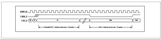
Figure 11 10M RMII Transmit Diagram
