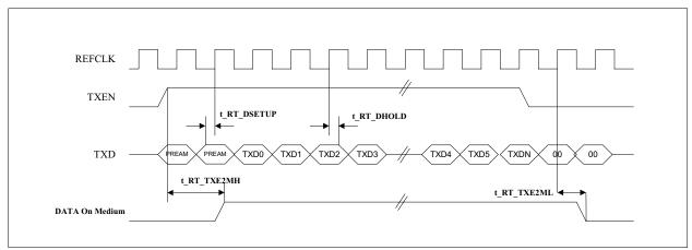
Figure 28 RMII Transmit Timing
