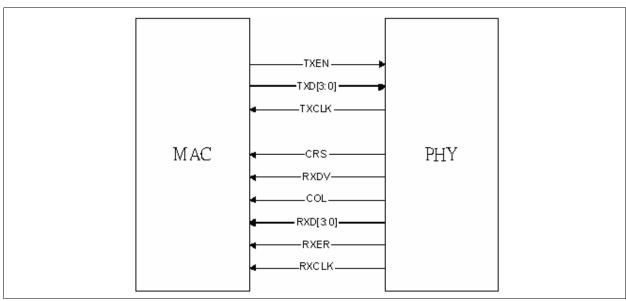
Figure 12 MII Signal Diagram
