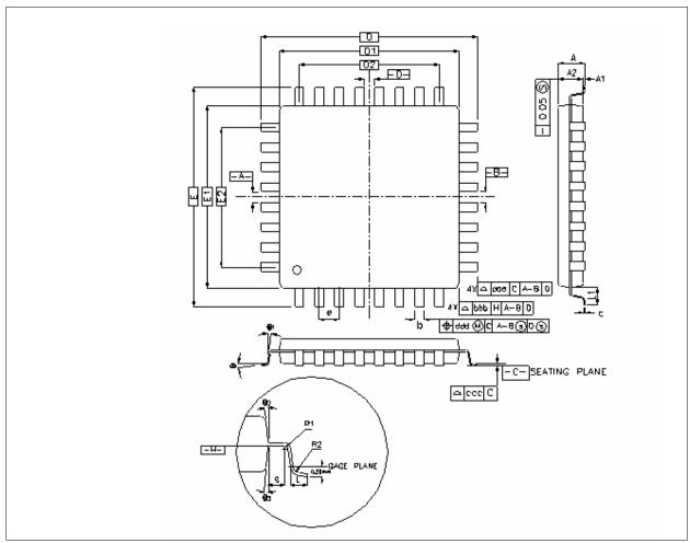
Figure 38 ADM7001,Low Profile Quad Flat Package (LQFP)
