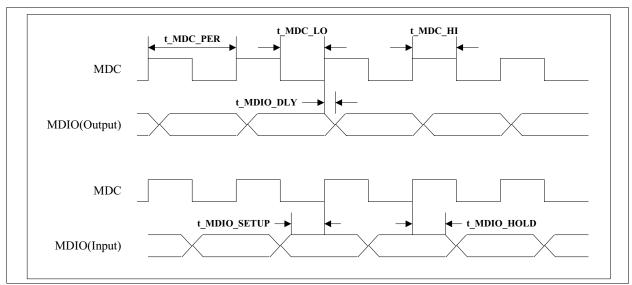
Figure 36 Serial Management Interface (MDC/MDIO) Timing
