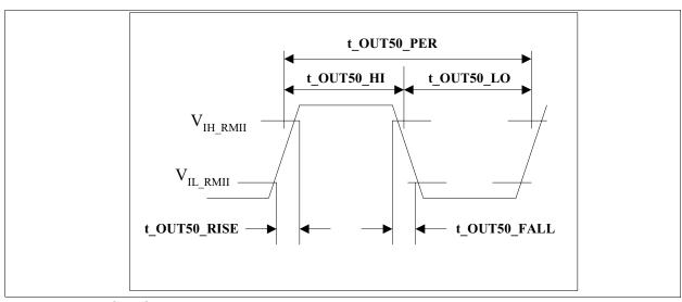
Figure 27 REFCLK Output Timing
