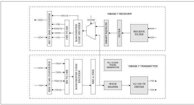
Figure 4 10Base-T Block Diagram and Data Path
