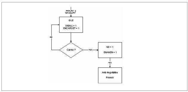
Figure 23 Medium Detect Power Management Flow Chart
