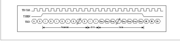
Figure 20 GPSI Transmit Diagram
