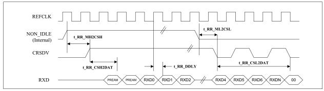
Figure 29 RMII Receive Timing
