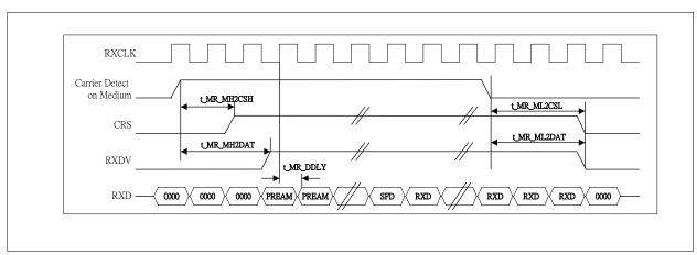
Figure 31 MII Receive Timing
