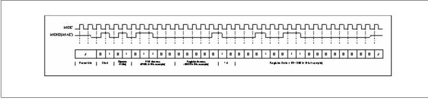
Figure 22 SMII Write Operation
