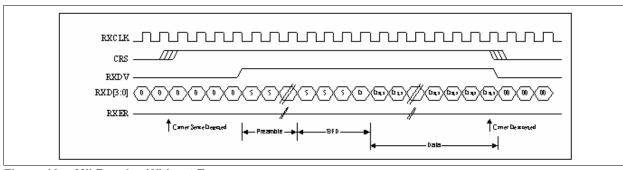
Figure 13 MII Receive Without Error
