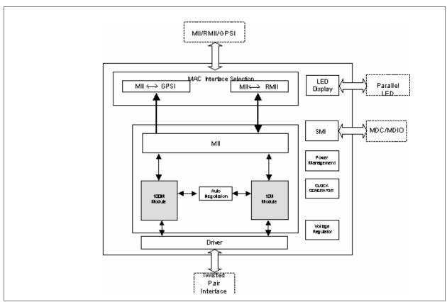
Figure 1 ADM7001 Block Diagram
