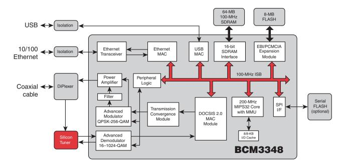
The **BCM3348** combines an RF receiver with an advanced QAM and S-CDMA demodular, an advanced QAM transmitter, a complete DOCSIS 2.0 Media Access Controller (MAC), a 200-MHz MIPS32<sup>™</sup> communication processor, a 16-bit, 100-MHz SDRAM interface, 10/100 Ethernet MAC with integrated transceiver and MII Interface, and a medium-speed USB 2.0 controller with integrated transceiver.
