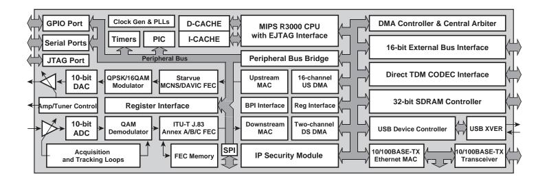
The Broadcom **BCM3350** represents a new level of costreduction for DOCSIS/EuroDOCSIS cable modems. Key modules integrated in the **BCM3350** include:
