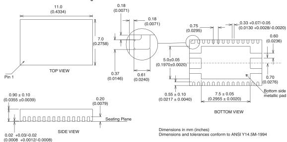
NOTE: For optimum solder joint size, MLP package printed circuit board lands should extend no more than 0.05 mm past the chip post on the short sides, and no more than 0.025 mm past the chip posts on the long sides.
