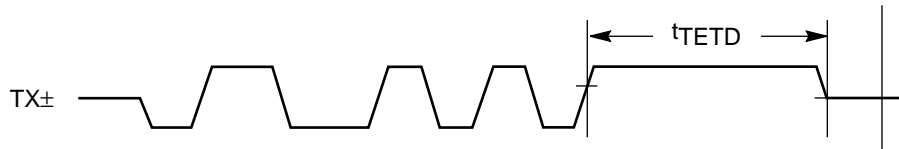
Figure 55 10 Mbps Transmit (TX±) Timing Diagram
