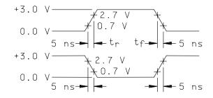
MEASUREMENTS: ALL CIRCUIT DELAYS ARE MEASURED AT THE +1.5 V LEVEL OF INPUTS AND OUTPUTS, UNLESS OTHERWISE SPECIFIED
