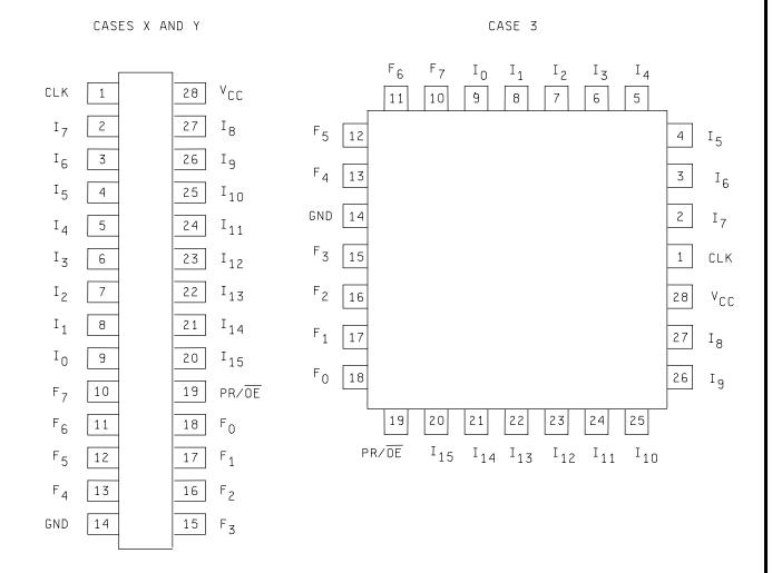
FIGURE 1. Terminal connections.
