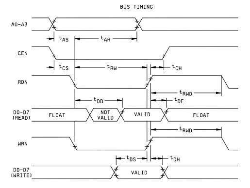
FIGURE 4. Timing waveforms and test circuits.
