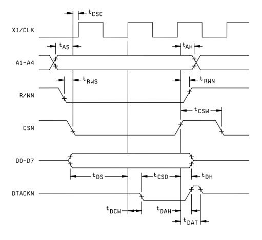
FIGURE 4. <u>Timing waveforms and test circuits</u> - Continued.
