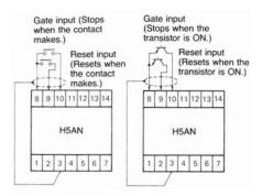
When connecting a solid-state circuit not of the open collector type to the gate or reset inputs as shown below, the voltage of the solidstate circuit (+V) should be 13 to 30 V, and the  $V_{\text{CE(S)}}$  of the transistor should be less than 3 V (the current that flows from either terminal 9 or 10 is approximately 10 mA). Moreover, it is essential that the circuit be ON for gate or reset input, and OFF when there is no input.
