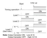
When a Load Operates with Contact Output
