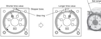
Note) The stoppers for the lower limit setting set ring and the upper limit setting set ring face the opposite directions.
