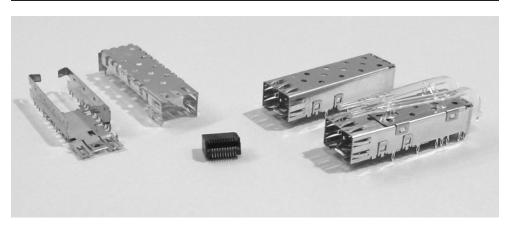
Tyco Electronics offers various termination options for SFP cages, including press-fit, wave solder and IR reflow compatible with tape and reel packaging. The connector is a reliable
