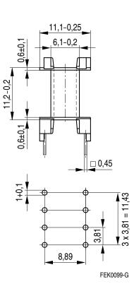
Hole arrangement View in mounting direction
