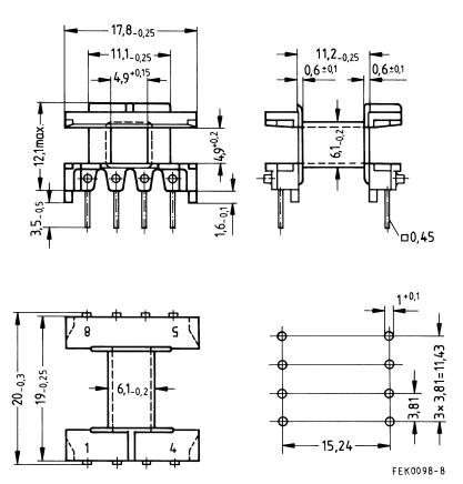
Hole arrangement View in mounting direction
