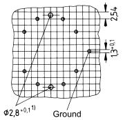
Hole arrangement View in mounting direction
