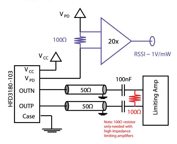
Optional RSSI implementation is shown in blue Optional  $100\Omega$  differential termination for high impedance limiting amplifiers is shown in red.
