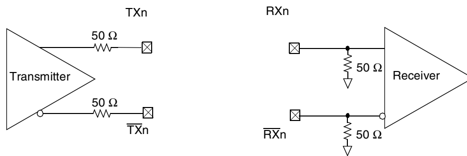
Figure 49. SerDes Transmitter and Receiver Reference Circuits
