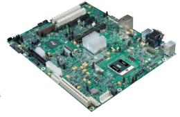
This platform enables outstanding instruction execution/watt while providing scalability with the Intel® Celeron® M and Intel® Pentium® M processors on 90nm process. This development kit features the Intel® Pentium® M processor 760° with Mobile Intel 915GM Express chipset, providing a high-performance, low-power solution for communications, industrial automation, point-of-service, and kiosk applications.
