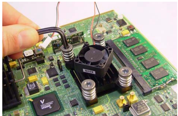
Figure 7-2. Loosen Allen screws
