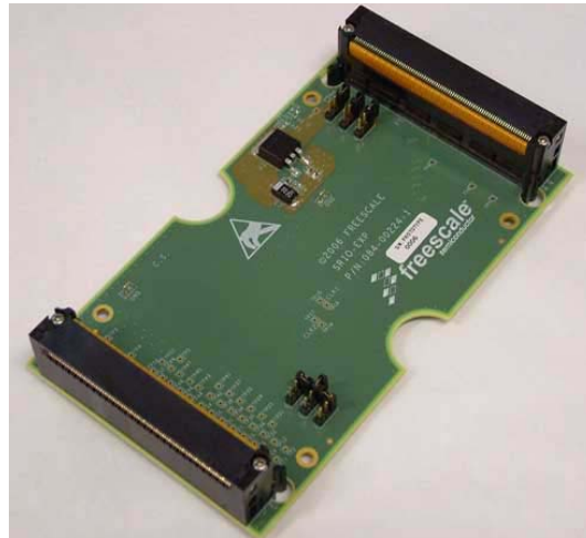
Figure 6-1. AMC Connecting Module
