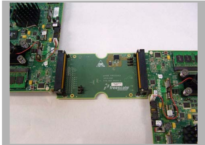
Figure 6-3. Two MSC8144ADS Boards Connected, Back-to-back
