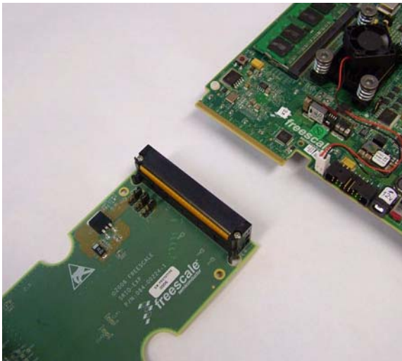
Figure 6-2. Fastening the AMC Module to the Edge Connector
