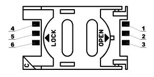
This is standard SIM card connector, to operate MOD-GSM-EDGE should have inserted valid SIM card for your operator network.
