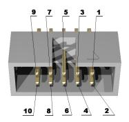
This connector allows connecting to other Olimex boards with UEXT connector.
