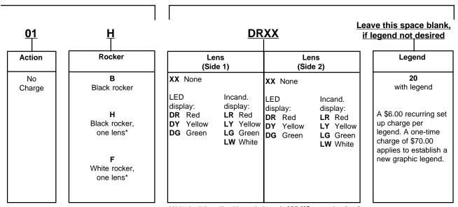
\* Lighted switches with solder terminals require MML93R receptacle to install lamps or LEDs.
