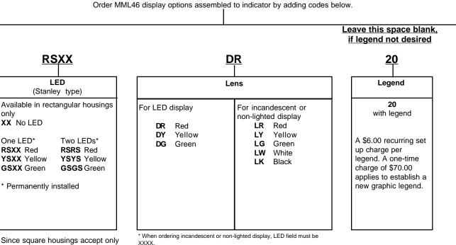
Since square housings accept only one LED, only a two-character LED code is necessary. For example: MML46HR0**XX**DY or MML46HR0**RS**DY
