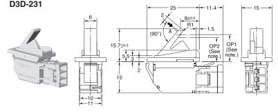
Note: The dimensions OP1 and OP2 apply to the D3D-211 only. The D3D-221 and D3D-231 are SPST-NC and SPST-NO respectively and so therefore have only one corresponding dimension here (OP).
