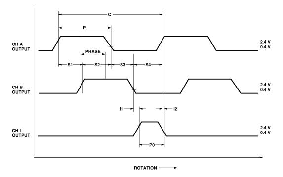
Waveforms for Encoders without Line Drivers.
