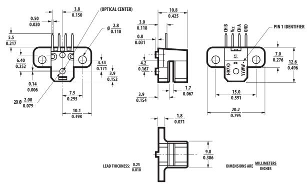
Mounting Option #51 – Screwmount (Baseplane Mounting)
