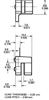
Mounting Option #50 - Standard (Baseplane Mounting) Contact Factory for Detailed Package Dimensions
