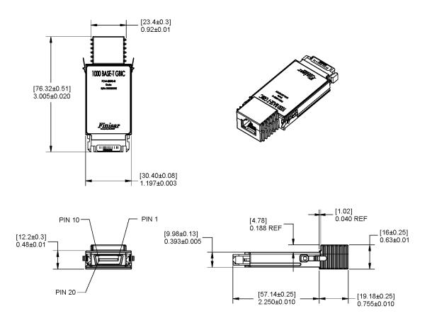
Figure 1. FCM-8520/8521-3 mechanical dimensions
