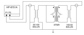
5. Crosstalk Attenuation — In the dual packages, which contain transmit and receive transformers side by side, sufficient crosstalk attenuation is achieved by the inherent characteristics of the toroid cores as well as by their proper positioning. The crosstalk attenuation is typically 50 dB or better from 100 KHz to 10 MHz. This result was established with the test circuit shown below.
