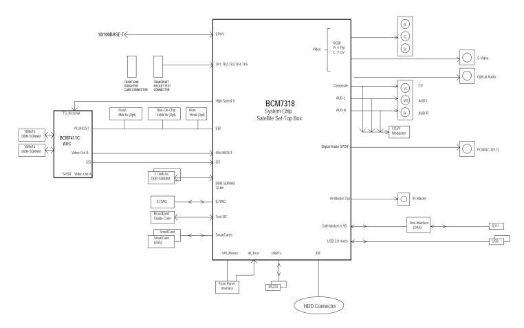
The Broadcom BCM97318AVC IP set-top box reference design is a complete hardware and software design based on the IP-STB-Chipset BCM7318 and BCM7411.
