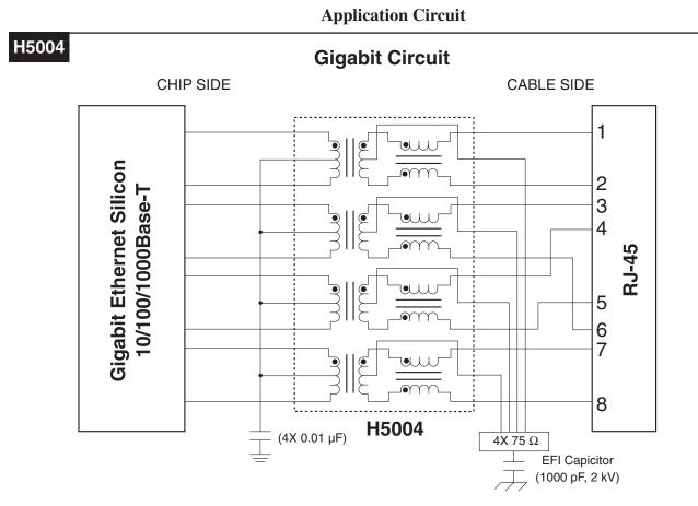
The above circuit is a simple interface for a gigabit transformer connectiong to both the Gigabit Ethernet silicon and the RJ-45 connector.
