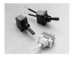
The D-Series toggle switches are single pole and have ratings up to 20 amps and 1-1/2 horsepower. These switches have a nylon toggle and base, and are also available with integrated wire leads.
