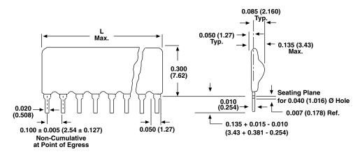
Pin #1 is extreme left-hand terminal on side with marking.
