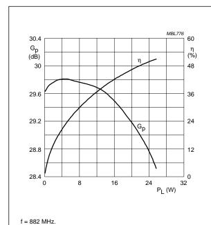
Fig.6 CW gain power and efficiency as functions of load power; typical values.
