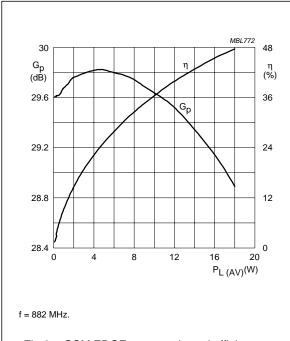
Fig.2 GSM EDGE power gain and efficiency as functions of load power; typical values.
