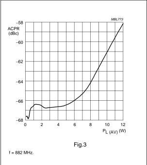
Fig.3 GSM EDGE ACPR at 400 kHz as a function of load power; typical values.
