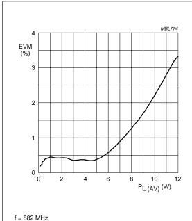
Fig.4 GSM EDGE rms EVM as a function of average load power; typical values.
