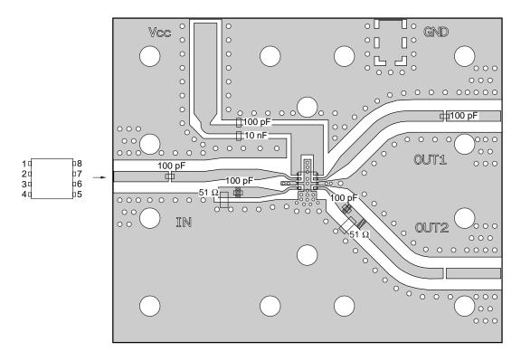
**Remarks 1.**  $33 \times 21 \times 0.4$  mm double-sided copper-clad polyimide PCB
