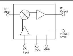
wireless communications such as cellular, PCS, and 900 MHz cordless phones. Operating on a 3 volt supply, this IC is ideally suited for hand held portable designs.
