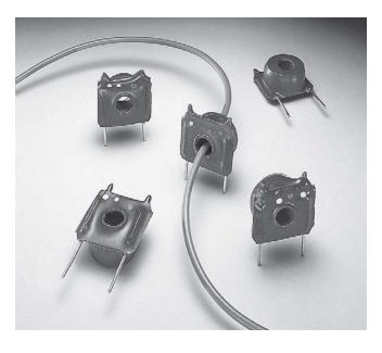
This Coilcraft current sensor is intended for measuring current from 1 to 10 A rms. The sensor functions as the encapsulated secondary of a current transformer, while the conductor carrying the current to be measured serves as the "one turn primary." Sensitivity may be enhanced by increasing primary turns.
