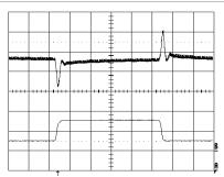
Output voltage response to load current step-change (10-30-10 A) at: Top trace: output voltage (200mV/div.). Bottom trace: load current (20 A/div.). Time scale: (0.1 ms/div.).
