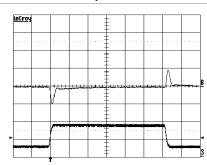
Output voltage response to load current step-change (3-9-3 A) at: Tp1 =+25°C,  $V_1$  = 53 V. Top trace: output voltage (500mV/div.). Time scale: (0.1 ms/div.).
