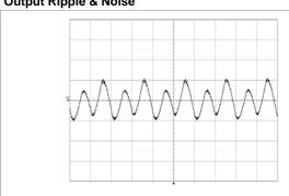
Output voltage ripple at:  $T_{p1} = +25^{\circ}C$ ,  $V_{I} = 53$  V,  $I_{O} = 60$  A resistive load.
