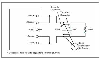
Output ripple and noise test setup
