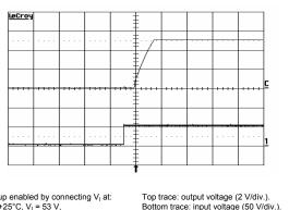
Start-up enabled by connecting  $V_l$  at:  $T_{p1}$  = +25°C,  $V_l$  = 53  $V_r$ ,  $I_O$  = 28 A resistive load.
