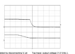
Shut-down enabled by disconnecting  $V_{l}$  at:  $T_{p1} = +25^{\circ}C$ ,  $V_1 = 53 V$ ,  $I_0 = 60 A$  resistive load.
