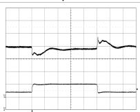
Output voltage response to load current step-change (15-45-15 A) at: Bottom trace: load current (50 A/div.).  $T_{p1} = +25^{\circ}C, \ V_{l} = 53 \ V.$  Time scale: (0.1 ms/div.).
