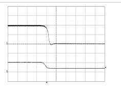
Shut-down enabled by disconnecting V<sub>I</sub> at:  $T_{p1}$  = +25°C, V<sub>I</sub> = 53 V,  $I_{O}$  =60 A resistive load.
