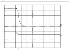
Shut-down enabled by disconnecting  $V_l$  at:  $T_{p1}$  = +25°C,  $V_l$  = 53 V,  $I_0$  = 40 A resistive load.
