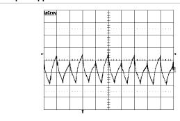
Output voltage ripple at:  $T_{p1}$  = +25°C,  $V_{I}$  = 53 V,  $I_{O}$  = 40 A resistive load.
