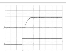
Start-up enabled by connecting  $V_l$  at:  $T_{p1}$  = +25°C,  $V_l$  = 53 V,  $I_O$  = 60 A resistive load.
