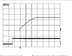
Start-up enabled by connecting  $V_l$  at:  $T_{p1}$  = +25°C,  $V_l$  = 53  $V_s$ ,  $I_O$  = 12 A resistive load.
