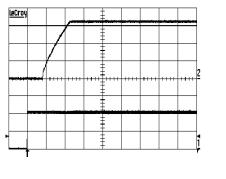
Start-up enabled by connecting  $V_l$  at:  $T_{p1}$  = +25°C,  $V_l$  = 53  $V_s$ ,  $I_O$  = 40 A resistive load.
