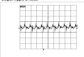
Output voltage ripple at:  $T_{p1}$  = +25°C,  $V_{I}$  = 53 V,  $I_{O}$  = 12 A resistive load.
