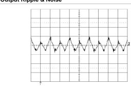
Output voltage ripple at:  $T_{p1} = +25^{\circ}C$ ,  $V_{I} = 53$  V,  $I_{O} = 60$  A resistive load.
