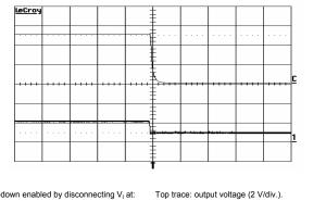
Shut-down enabled by disconnecting  $V_{l}$  at:  $T_{p1}$  = +25°C,  $V_{l}$  = 53 V,  $I_{O}$  = 28 A resistive load.
