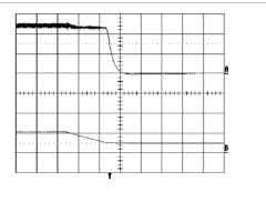
Shut-down enabled by disconnecting V<sub>I</sub> at:  $T_{p1} = +25^{\circ}C$ ,  $V_1 = 53 V$ ,  $I_0 = 30 A$  resistive load.
