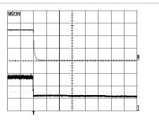
Shut-down enabled by disconnecting  $V_l$  at:  $T_{p1}$  = +25°C,  $V_l$  = 53 V,  $I_0$  = 12 A resistive load.
