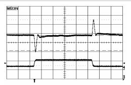
Output voltage response to load current step-change (7-21-7 A) at:  $T_{\rm p1}$  =+25°C,  $V_{\rm l}$  = 53 V.
