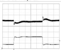
Output voltage response to load current step-change (15-45-15 A) at: Bottom trace: load current (20 A/div.).  $T_{p1} = +25^{\circ}C, \ V_{l} = 53 \ V.$  Time scale: (0.1 ms/div.).
