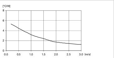
Thermal resistance vs. airspeed measured at the converter. Tested in wind tunnel with airflow and test conditions as per the Thermal consideration section.
