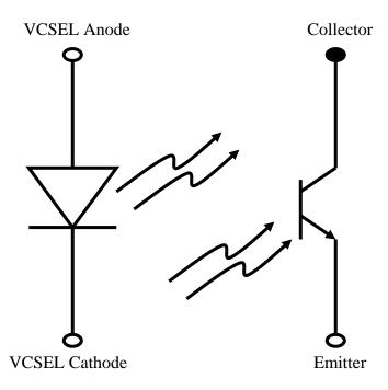
It is recommended in application that a  $100\text{-}1000\Omega$  load resistor be connected between the emitter and a negative power supply between 5 and 15V. The output can be read as the voltage across the resistor. Alternatively, the case can be connected to a power supply with the load resistor remaining connected to the emitter.
