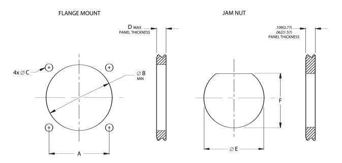
**Note 1:** Flange Mounting Dimensions ( $\emptyset$  B cutout and D MAX) listed only for back of panel mounting (MS27497 and MS27508).
