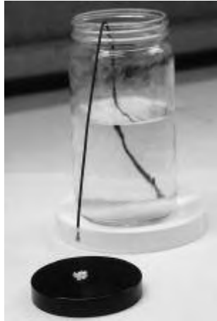
A salt deposit can be seen beneath the end of this 18-AWG, 19-strand wire. The other end of the wire has been immersed in salt water for 24 hours.
