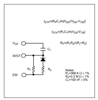
Figure 8 - Non-Symmetric Guard Time Circuit
