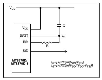
Figure 4 - Basic Steering Circuit
