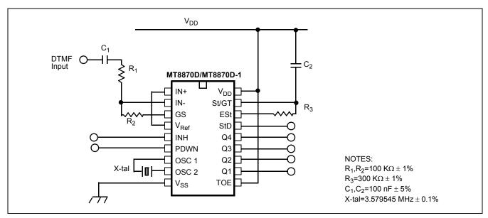
Figure 10 - Single-Ended Input Configuration
