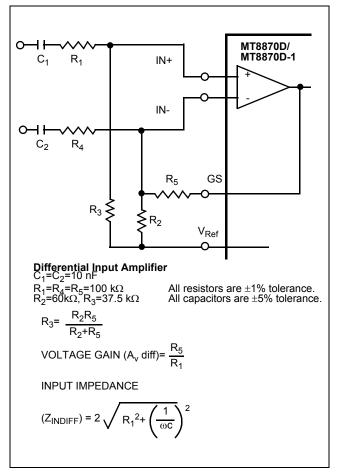
Figure 6 - Differential Input Configuration
