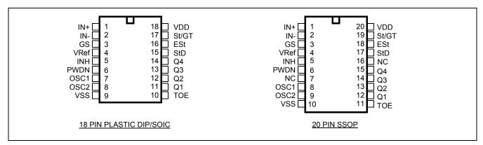
Figure 2 - Pin Connections
