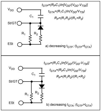
Figure 5 - Guard Time Adjustment
