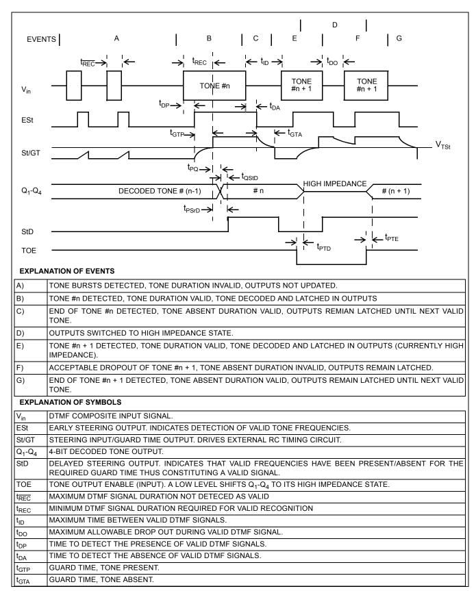
Figure 11 - Timing Diagram
