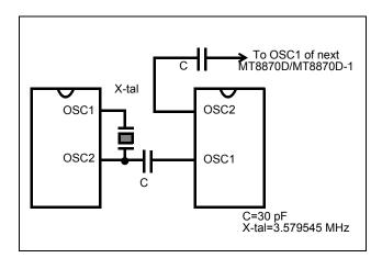
Figure 7 - Oscillator Connection
