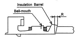
The dimension "R" of the declined insulation barrel is more than 0.5 mm.
