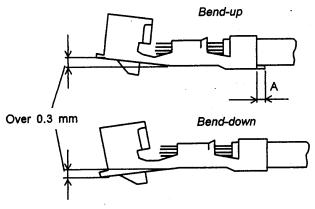
Based from the wire crimped portion, the bend-up amount or the bend-down amount of the mating tip is no less than 0.3 mm.
