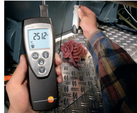
Temperature measurement of ductile materials with the fast-action penetration probe
