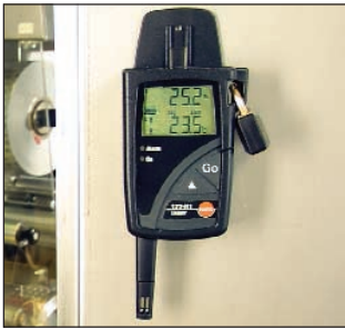
Wall holder, for quick attachment of logger to wall
