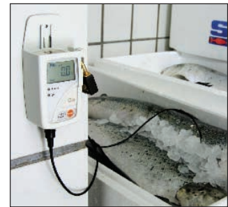
Simultaneous monitoring of product and air temperature e.g. in refrigerated rooms, during production, in containers etc.
