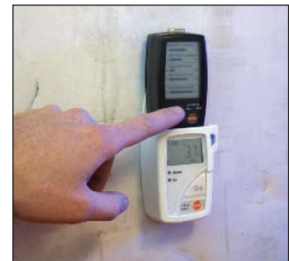
Collects data on-site, downloads and analyses centrally on PC. The high-performance data collector reads out approx. 400 readings/s.
