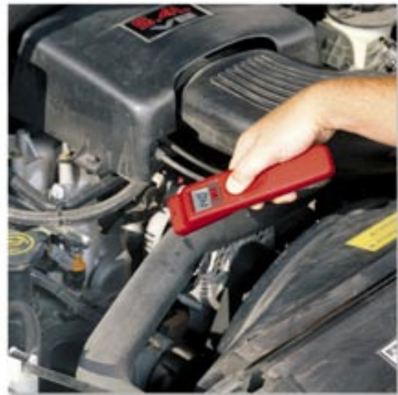
Check cylinder heads, heating and cooling systems, and scan radiators for blockage.
